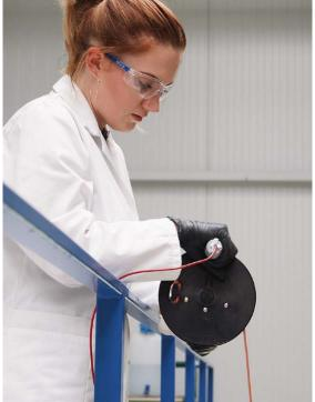
The Dipping Bottles are made of non-spark producing brass or stainless steel. In combination with an electrically conductive drum reel and a suitable lowering cable from Bürkle the danger of ignition due to accumulation of electrostatic charge is excluded.
