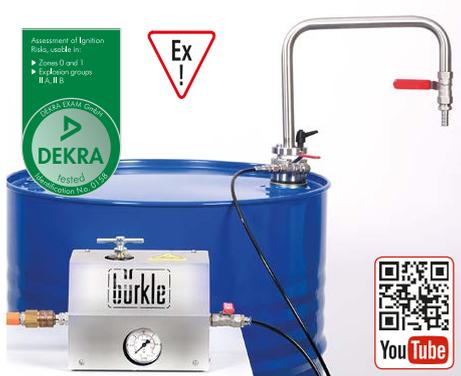
The withdrawal system can be used to dispense high-purity liquids quickly and without complications. An excess pressure is produced in the container with pressurised gas (compressed air or nitrogen), thereby pumping the liquid out of the tank. In this way, large amounts of hazardous media can also be safely dispensed and accurately metered. For use with media sensitive to oxygen or for
