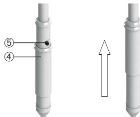
2. At the desired depth, pull back the instrument approx. 10 cm. Thereby, the sliding sleeve opens the filling opening.
