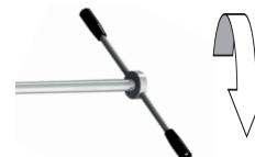
3. After approx. 5 rotations, the sampling chamber is filled.
