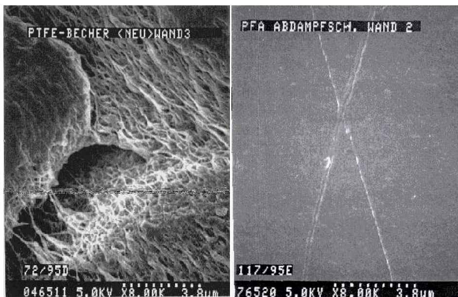
Fig. 1 SEM image of surface of a PTFE beaker (left) and a PFA evaporating dish (right). REM x8000, sample tilt 30°.
